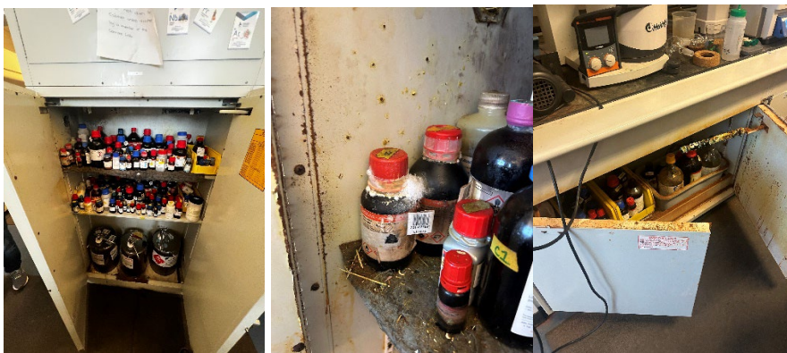
Photos: No segregation of incompatibles are seen. Some chemicals are in concerning states and possible time and chemical vapor release have led to corrosion of the cabinets.
