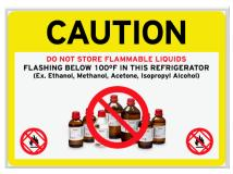
conventional/household refrigerators. For this reason, flammable materials with a flash point less than 100°F, if necessary to be stored below ambient temperature, must be stored in explosion-proof or flammable storage refrigerators.
