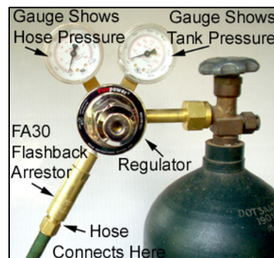
Figure 9. Regulators, Hoses, Tanks & Torch Connections 7
