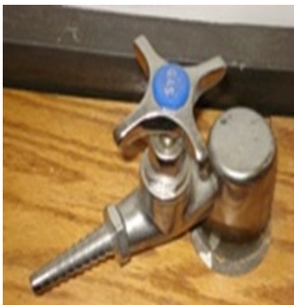
Turn valve clockwise to close To close, make sure lever is perpendicular to
