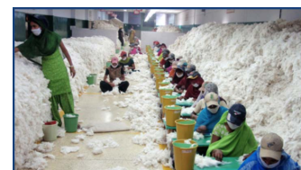
Pesticide and soil particles become trapped in cotton dust during the processing and spinning of cotton
