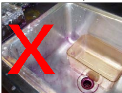
Stained sink due to drain disposal
